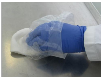
Figure 1: Wiping device gripped through a plastic bag
